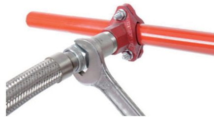
Fig.3: Tightening the hexagon nut and inlet pipe to a maximum of 20N·m(15ft-lbs), and check that the sealing ring is in right condition. Do not over tighten the nut. Excessive torque may damage the sealing ring.
